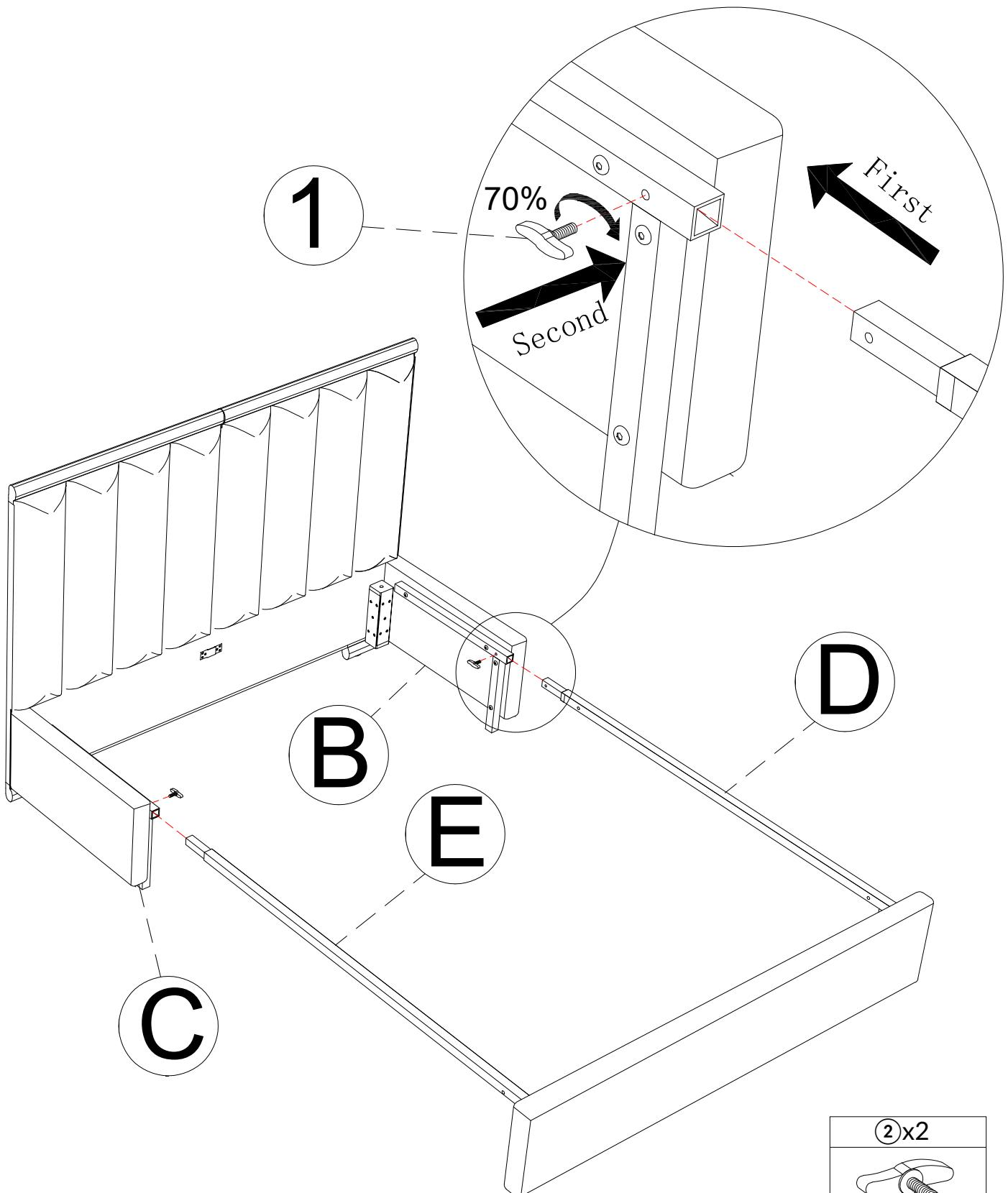
First, Tighten the threaded rod 70%
