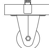
A diagram of a fixed caster with a rectangular base plate and a circular wheel.                           |
