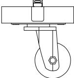
A diagram of a swivel caster with a rectangular base plate and a circular wheel.                           |
